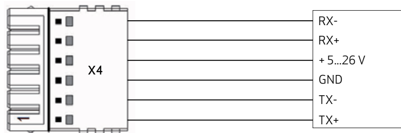
Fig. 9: Connector X4 pin assignment and external interface
