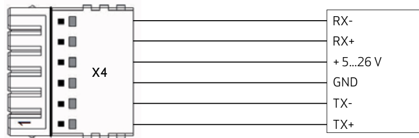
Fig. 9: Connector X4 pin assignment and external interface
