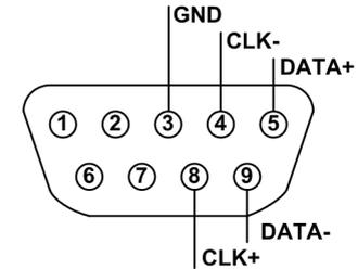
Figure 1.1 Pin assignment of SSI Encoder Simulation
