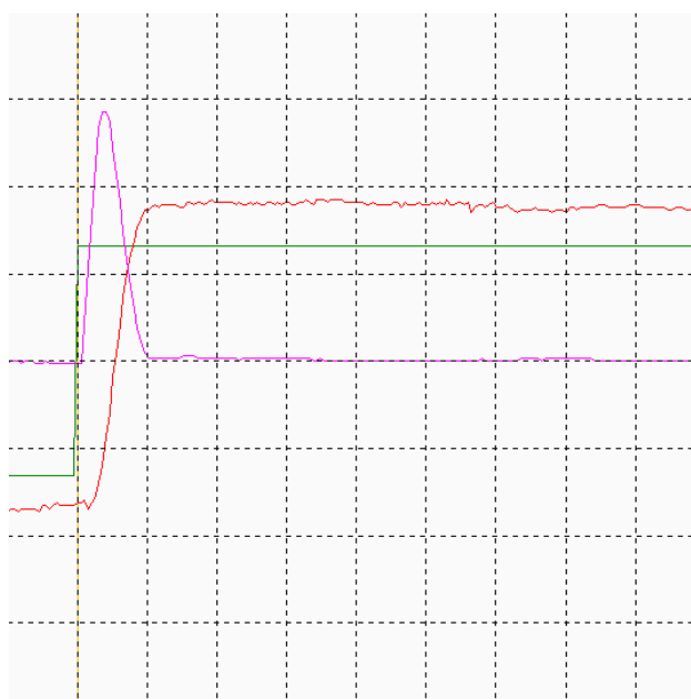
Figure 4-9 CSA Step Response with Maximum Velocity Loop Gains
