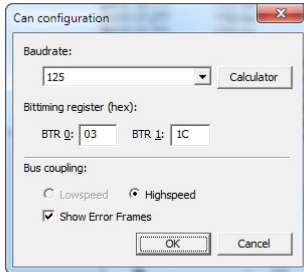
Fig. 2-5: Configuration dialog of the CAN controller
