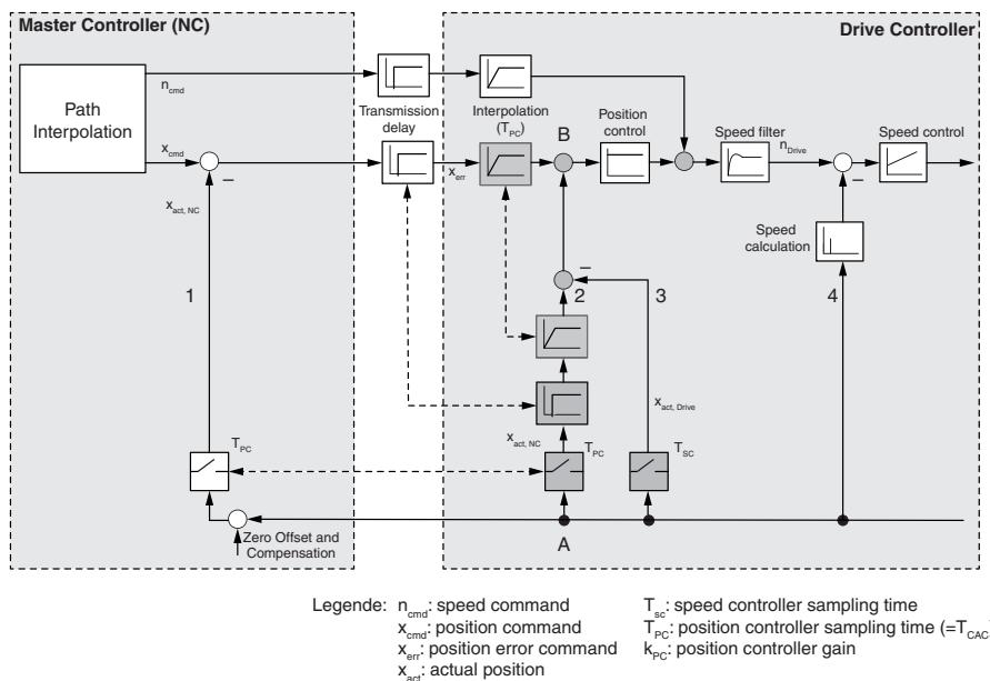
Figure 10.8 Position control with Dynamic Servo Control
