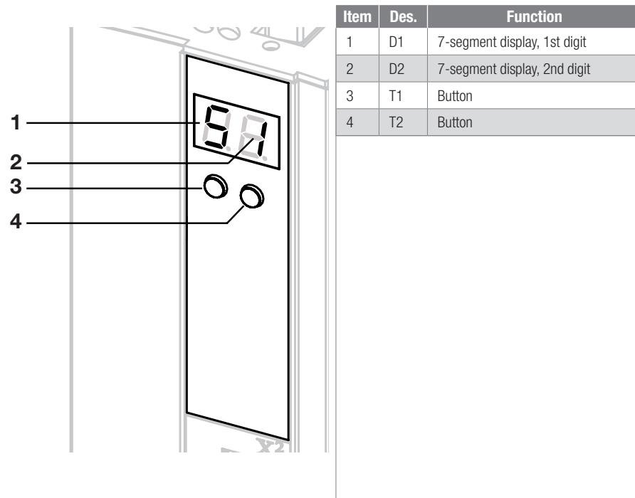
Table 4.3 Items on the integrated control unit on the MSD Servo Drive
