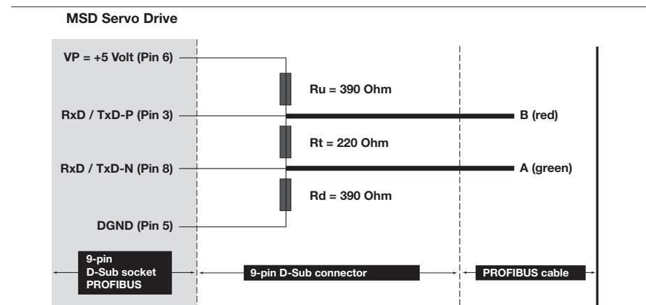
Figure 6.1 Bus termination in the 9-pin D-Sub connector
