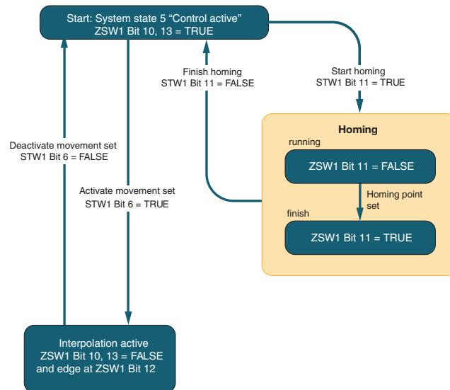
Figure 10.6 Position control (interpolating mode - PROFINET)
