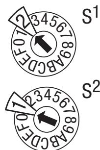
Figure 4.2 Coding switches for PROFIBUS address
