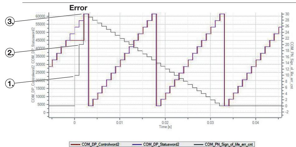
Figure 8.4 3 sign of life errors triggered
