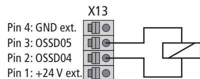
Figure 7.13 Brake driver circuit example 2
