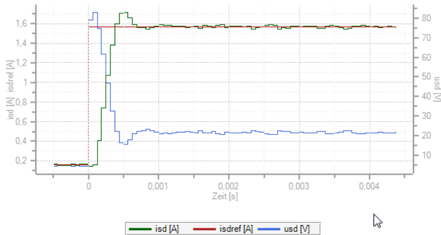
Fig. 7.6: Current controller optimization
