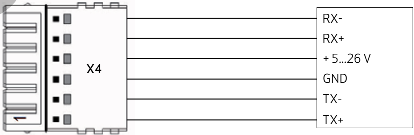
Fig. 9: Connector X4 pin assignment and external interface
